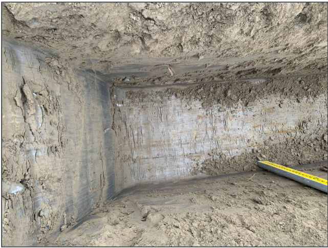
Fig 5. TP04 - fill/silt contact 0.6 m.
